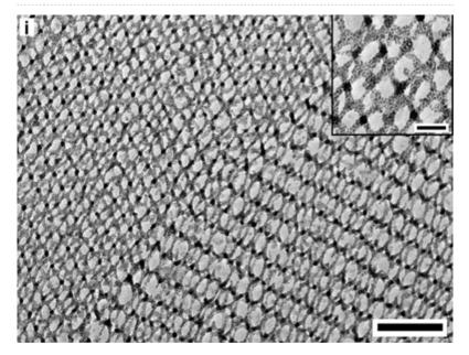
from the Japan Science and Technology Agency used electron tomography to map the location of every single particle in the samples, which then could be compared with theoretical predictions. The result is a comprehensive set of design criteria that could lead to readying these particle networks for larger scale solution processing.
